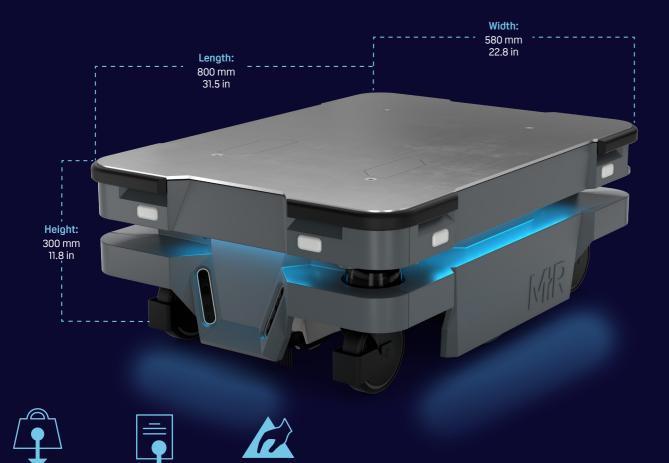
The MiR250 has a small footprint of just 580 x 800 mm and stands at a mere 30 centimeters tall. Despite its size, it can effortlessly handle up to 250 kg, moving along at 2 meters per second. This agility sets it apart from all other AMRs on the market, making it exceptionally adaptable to demanding environments.
